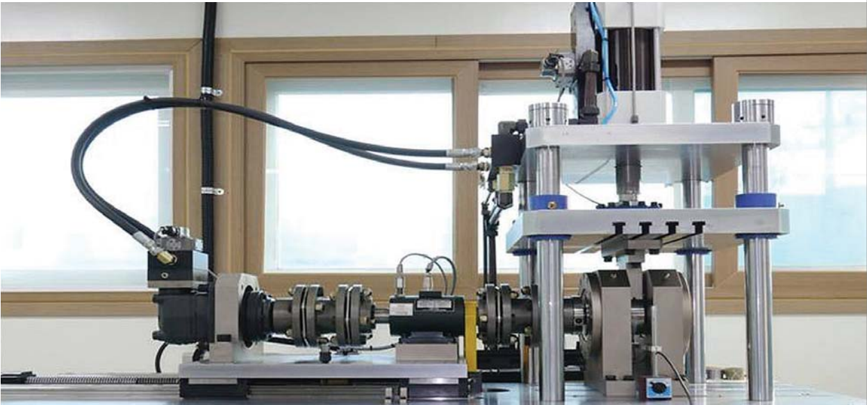
Fig 2. Friction and wear test rig at SOLTRI lab.
